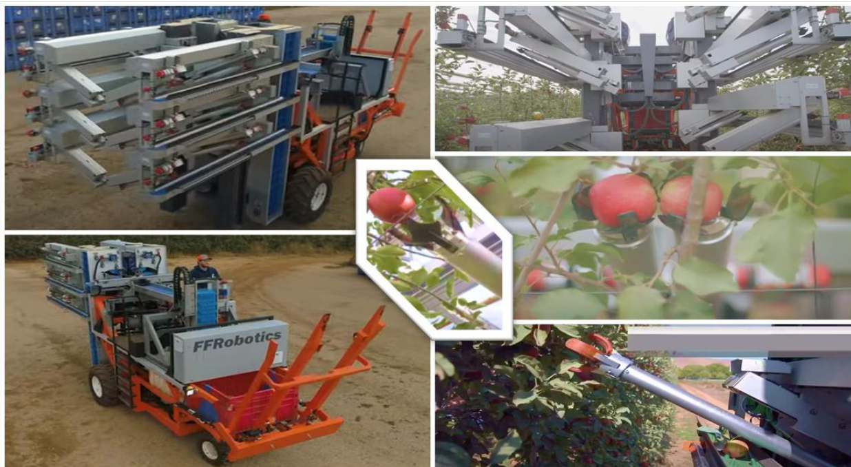
Figure 42. Multiple-arm apples' harvesting robot
